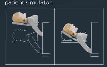
In order for both small as well as large students to be able to take up an ergonomic treatment position, the simulator has a wide range of options for adjusting the height and tilt.
